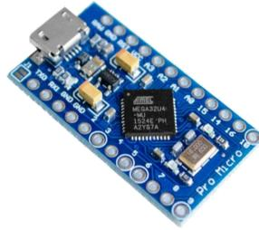
Figura 3.8: Arduino pro micro
