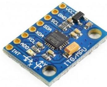
**Figura 3.5** Sensor MPU6050.
