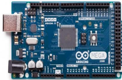
Figura 3.8: Arduino Mega 2560
