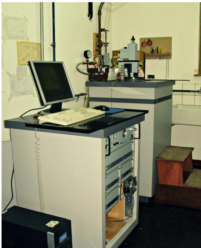
Figura 2.9. Magnetómetro SQUID Quantum Design MPMS 5S.
