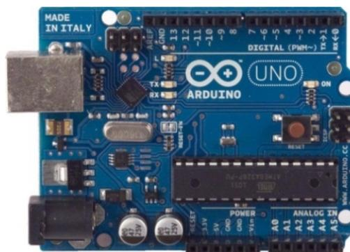
Figura 5.3 Tarjeta Arduino Uno
