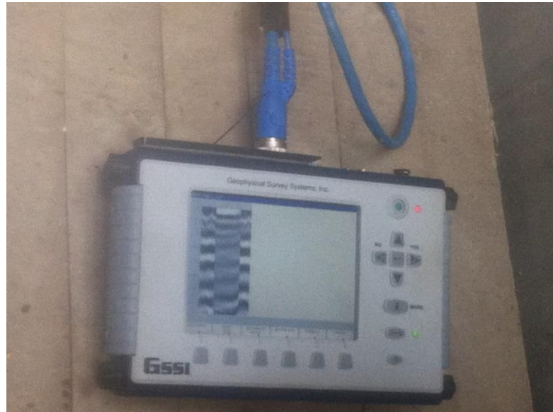
Figura N° 15. Ground Penetrating Radar Equipment (Fuente: propia).
