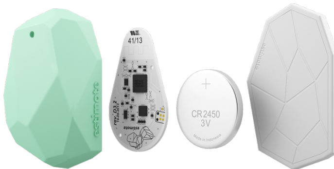
Figure 4.2 BLE beacon. (Taken from www.estimote.com )
