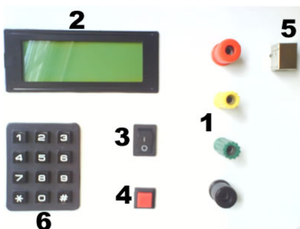
Figura B.2: Panel de control
