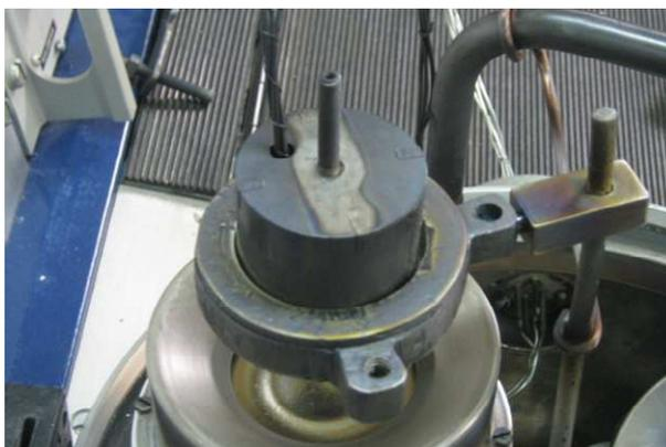
**Figura 24.** Horno calefactor
