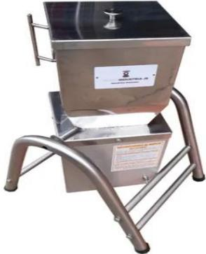
A stainless steel industrial blender with a large hopper on top and a motor base on a four-legged stand. It has a tilting mechanism for easy emptying.                                                                                                                                                                 |
