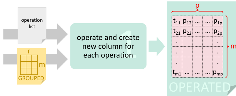
Figure C.5 Column operation process.
