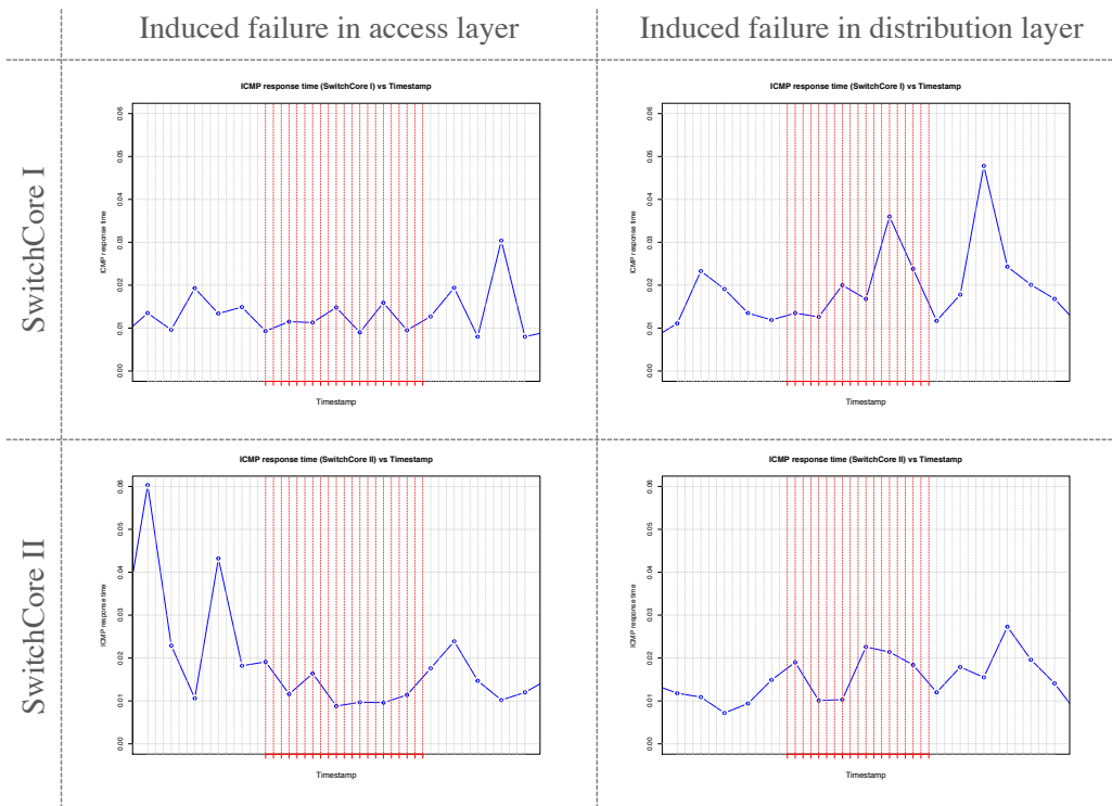
Figure 5.2 ICMP_response_time parameter behavior before, during, and after the failure. The failure time interval is indicated in red.
