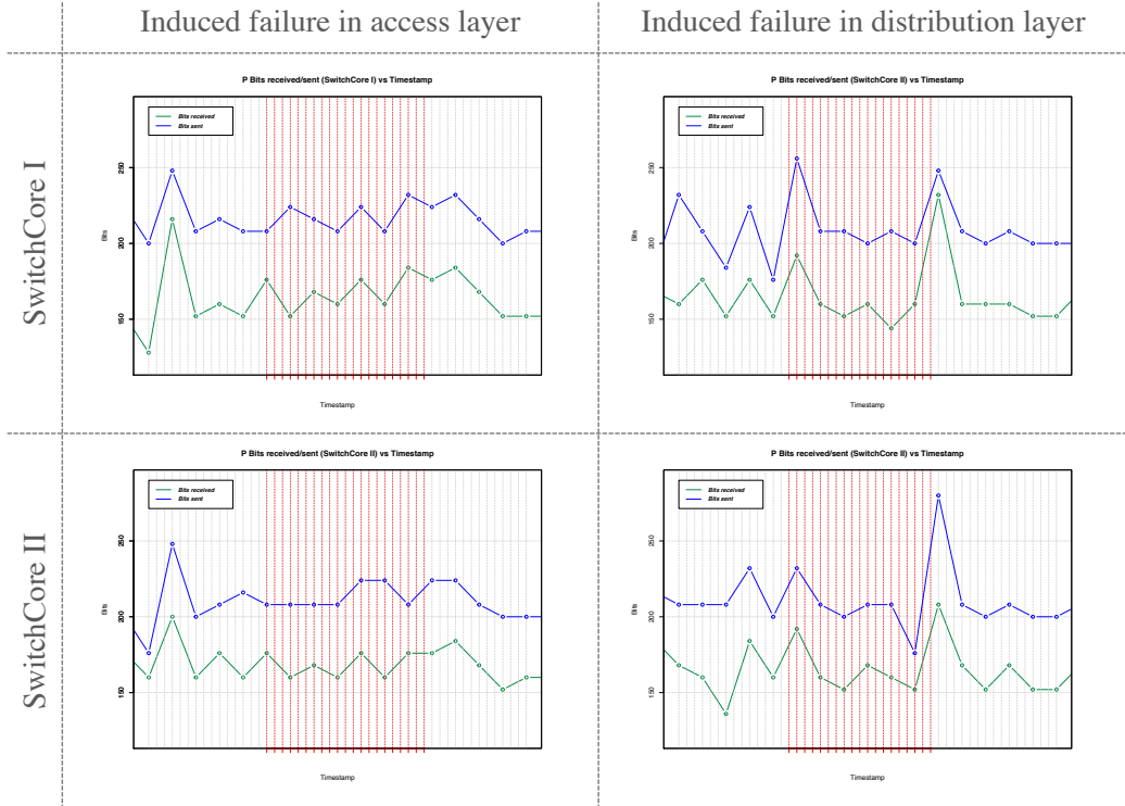
Figure 5.3 P_Bits_received and P_Bits_sent parameters behavior before, during, and after the failure. The failure time interval is indicated in red.
