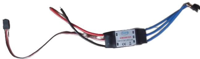
**Figura 2.2:** Electronic Speed Controller de 30A.
