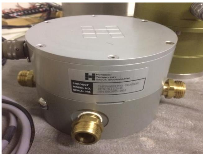
**Figura 12.** Sensor Hyperion Technology Group Slad, G., & Merchant, B. (2021). Evaluation of Low Cost Infrasound Sensor Packages. <https://doi.org/10.2172/1829264> [25].
